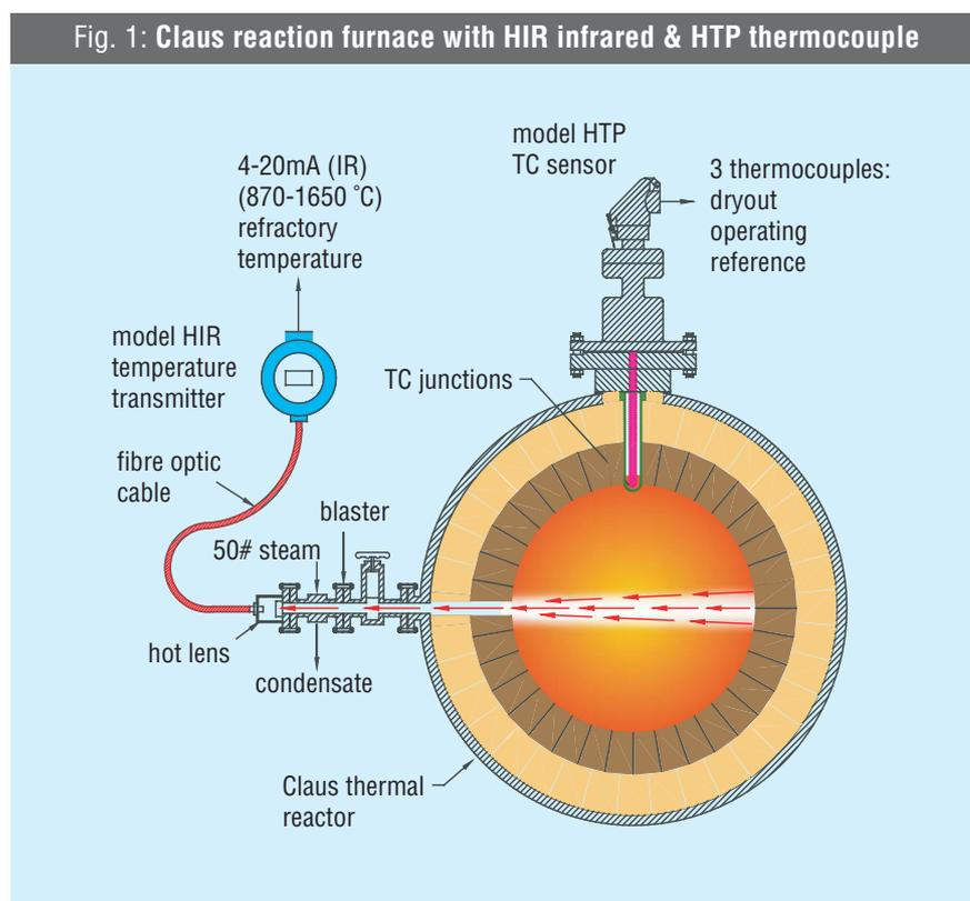
ceramic; the other is installed in a conventional manner with the junction protruding into the thermowell. In the unlikely event of a failure of the purged thermowell, the corrosive gases would attack the protruding element, whereas the encased one would be protected for an extended period of time. The corrosion would cause the signal to begin to drop relative to the actual temperature. The encased element would continue to provide an accurate signal. The disparity between
