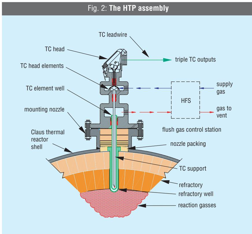
internal passages of the thermocouple. A slight elevated backpressure of the flush gas is maintained by the use of a flow meter equipped with a flow control valve located at the purge outlet. The purge function is most easily accomplished with the use of a convenient "flush gas" control station equipped with the pressure regulator, filter, drip well, flow meter and valve.
