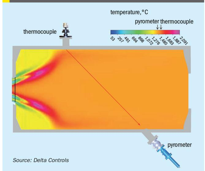
Fig 5: Side by side pyrometer calibration
