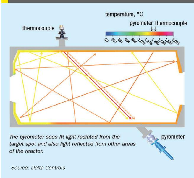
Fig 3: CFD model: the burner zone of a Claus thermal reactor with the pyrometer aimed directly at the thermocouple
