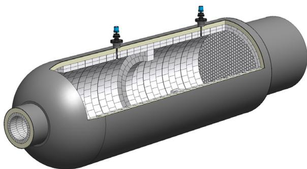
**Figure 1.** Thermocouples placed two-thirds to three-quarters from the burner to choke ring in zone 1 and from the choke ring to tube sheet ferrules in zone 2.
