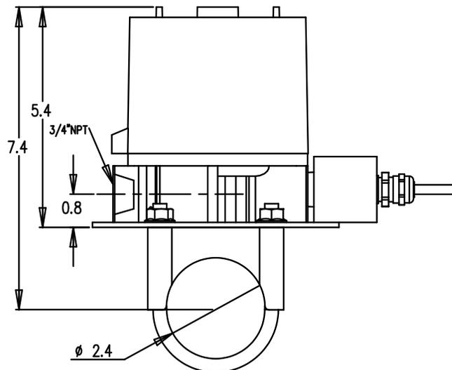
Figure 13 - Dimensions – Electronics Housing
