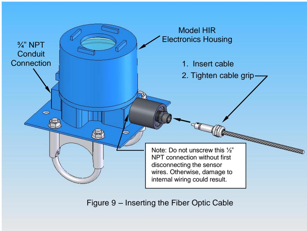
Figure 9 – Inserting the Fiber Optic Cable
