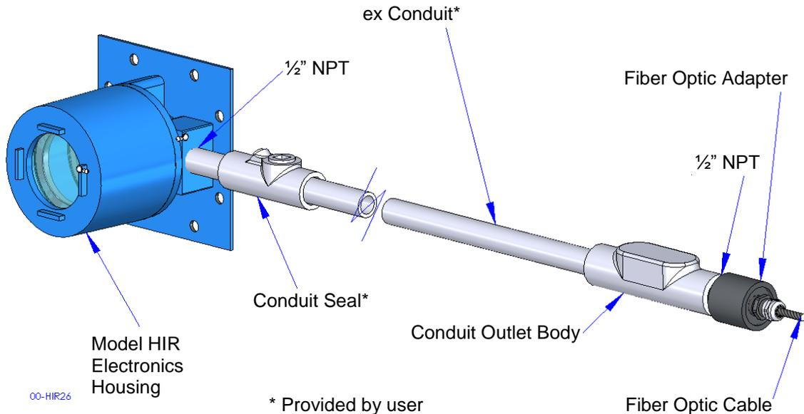
**Figure 6 Typical Installation of Remote Fiber Optic Adapter**
