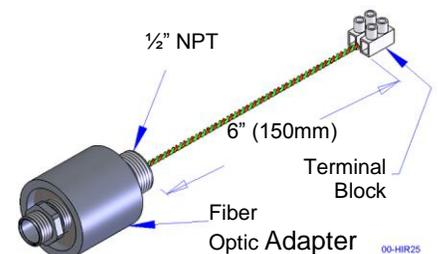
Figure 5 Fiber Optic Adapter
