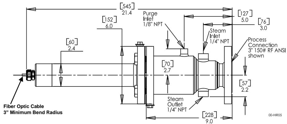
Figure 12 - Dimensions – Hot Lens Assembly
