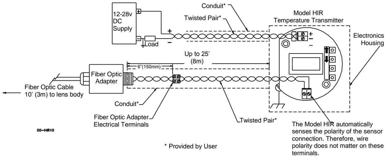
**Figure 8 Typical Wiring - Remote Sensor, option RS**
