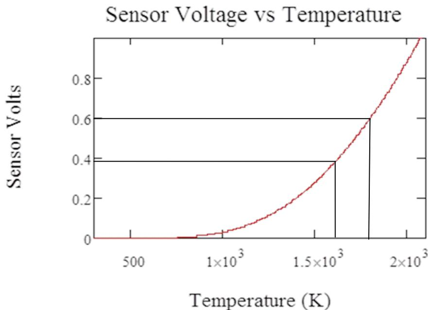
Figure 4 Typical Sensor Output vs. Temperature in a Pyrometer.
