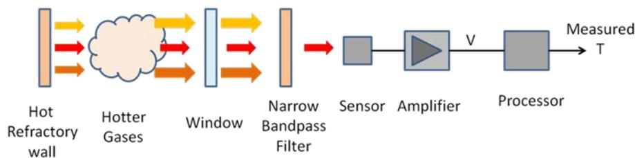
Figure 3 Schematic Representation of a Practical Single-Color Pyrometer
