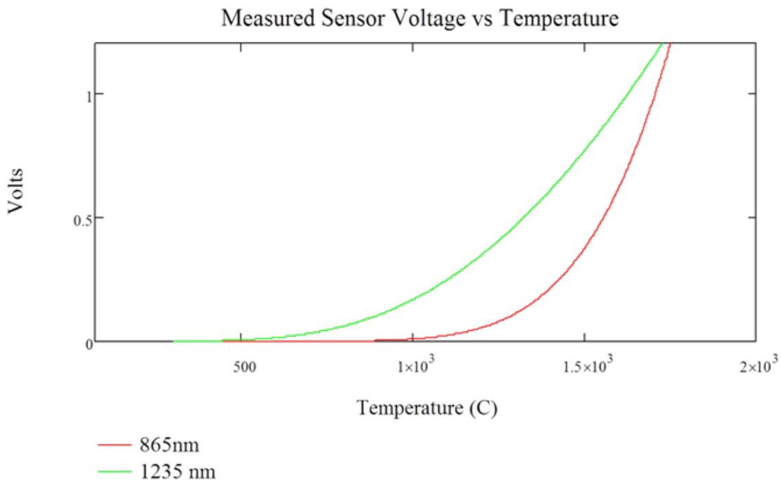
**Figure 6 Sensor Output vs. Temperature at Two Different Operating Wavelengths**
