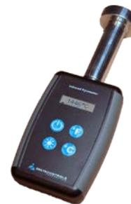
**Figure 9. Handheld two-color pyrometer can accurately read refractory temperature through partially clouded sight glass.**
