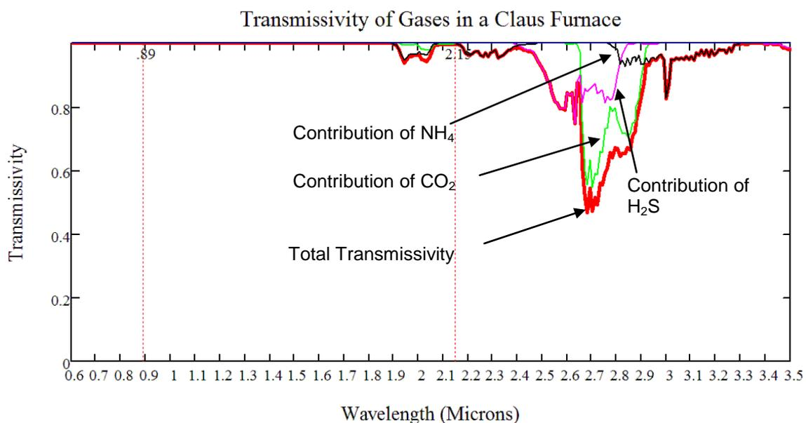
**Figure 11 Transmissivity of gases near the burner**
