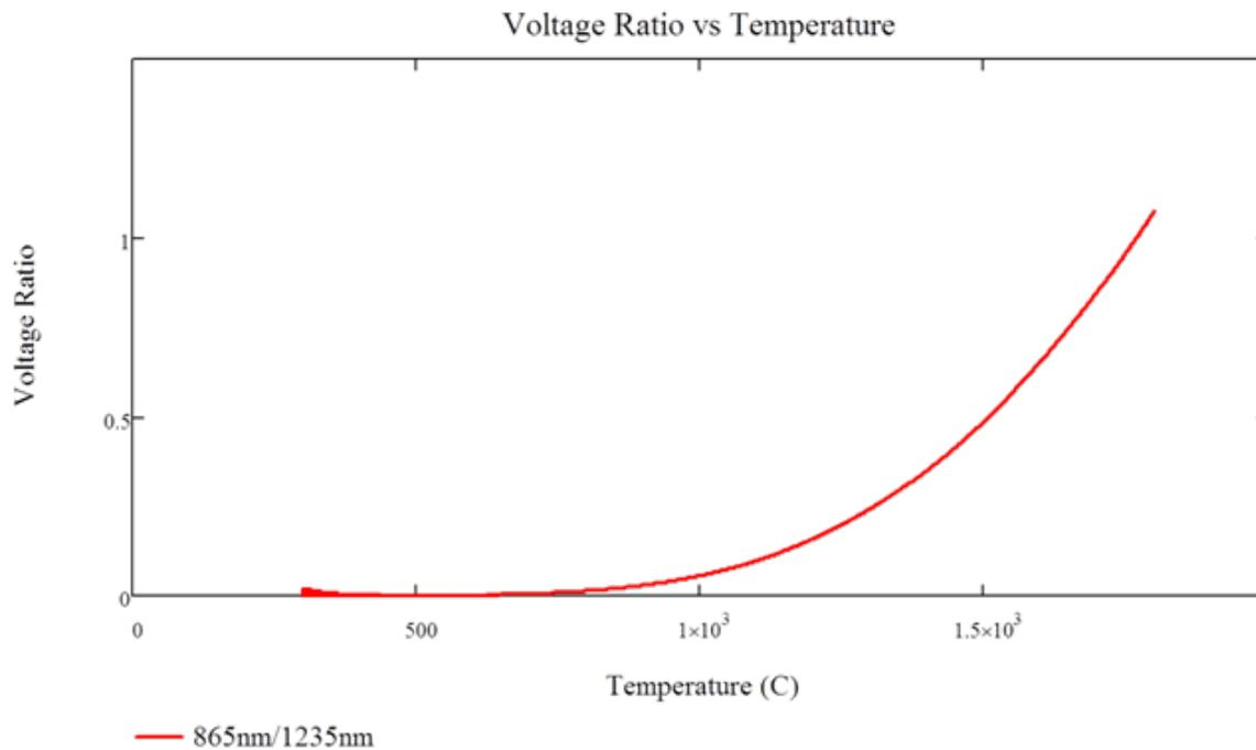
Figure 8 Sensor Output Ratio vs. Temperature
