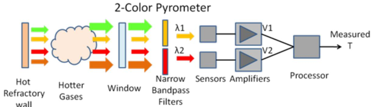
**Figure 5 Schematic of a Two-Color Pyrometer**
