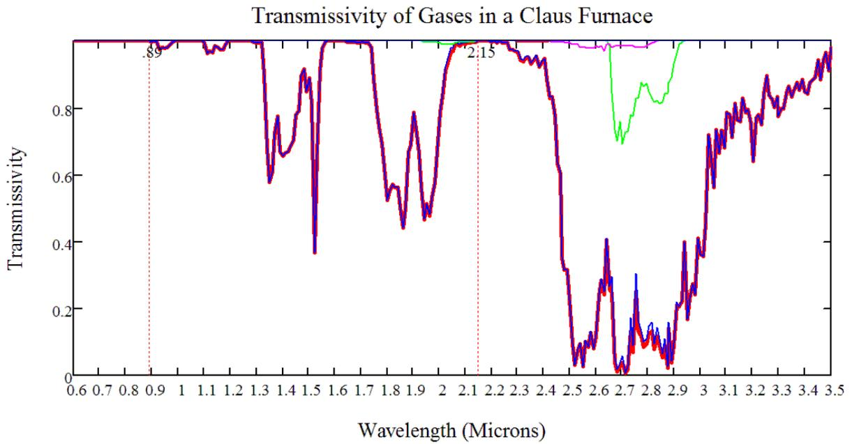
Figure 12 Transmissivity of gases near the tube sheet
