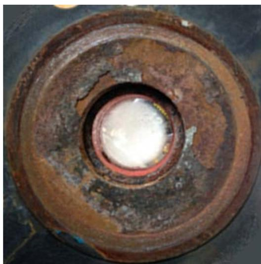
**Figure 1 Sulfur deposits on a pyrometer viewport window**
