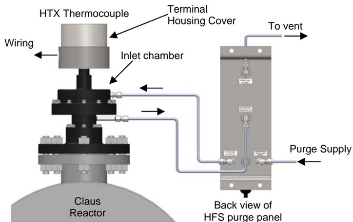
Under normal conditions of operation, the purge pressure should be set at least 5 PSIG (0.3 barg) above the max operating pressure of the reaction furnace. The flow rate should be set and maintained at approximately 0.2 to 0.4 scfh (5-11 lph). The exact rate is not important, only that some purge gas is always flowing through the thermocouple. Excessive flow will "cool" the thermocouple and cause inaccurate readings.
